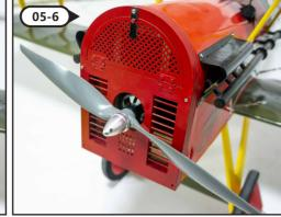
结合05-4,05-6两个步骤,根据马达尺寸调整马达座位置,调整好后用环氧胶粘固马达座。 In combination with steps 05-4 and 05-6, adjust the position of the motor base according to the size of the motor, and then use epoxy adhesive to fix the motor base.
