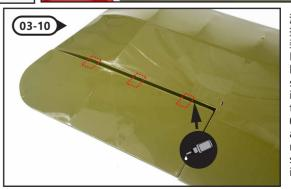
注意:上下机翼舵面均按03-9、03-10步骤安装,左右相同安装。 Note: The upper and lower wing control surfaces shall be installed according to steps 03-9 and 03-10. and the left and right wing control surfaces shall be installed the same.
